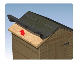
Remove the old roofing felt and remove the old fixing nails using a claw hammer or pincers.
