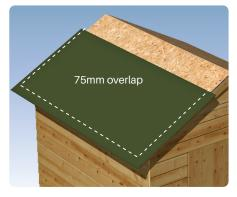
Cut each strip of felt so that it overhangs the edges of the roof by 75mm. Place the first strip of felt at the lowest part of the roof so that it overhangs the eaves by 75mm. Fix in position by nailing the top edge of the felt with 13mm galvanised clout nails at 500mm centres.
