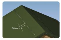
With the capping strip in position nail the lower edges at 50mm intervals. Carefully fold over the ends and secure with nails.
